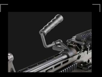
PZD 556 MK2 uses a quick change fluted barrels that improve the heat dissipation allowing the operator to sustain the operator of the machine gun for longer period of time without changing the barrel. Barrel comes with adjustable front sight and are zeroed identically to ensure there is no change in ballistics when swapped.
