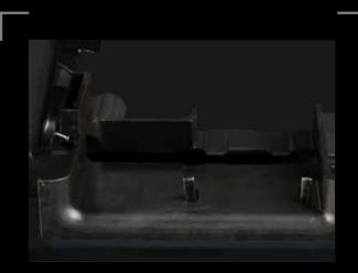
Modified feet tray with two retaining paws that hold the belt on the feed tray under any circumstances. This feature adds significant improvement when reloading or operating with NVGs.
