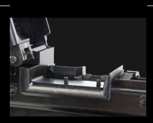
Modified feed tray with two retaining paws that hold the belt on the feed tray under any circumstances. This feature adds significant improvement when reloading or operating with NVGs.
