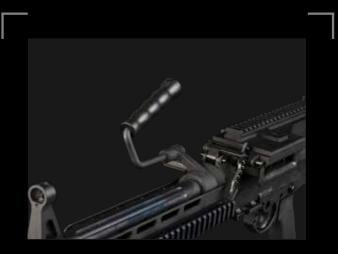
PZD 162 Mk1 uses a quick change flueted barrels that improve the heat dissipation allowing the operator to sustain the operator of the machine gun for longer period of time without changing the barrel. Barrel comes with adjustable front sight and are zeroed identically to ensure there is no change in ballistics when swapped.
